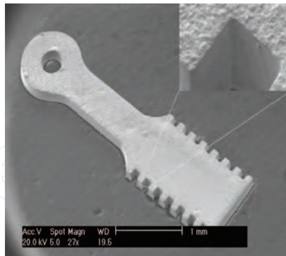
Fig. 15. A micro Ni-Al 2 O 3 piston electroformed from a bath containing 7g/l Al 2 O 3 particles.
