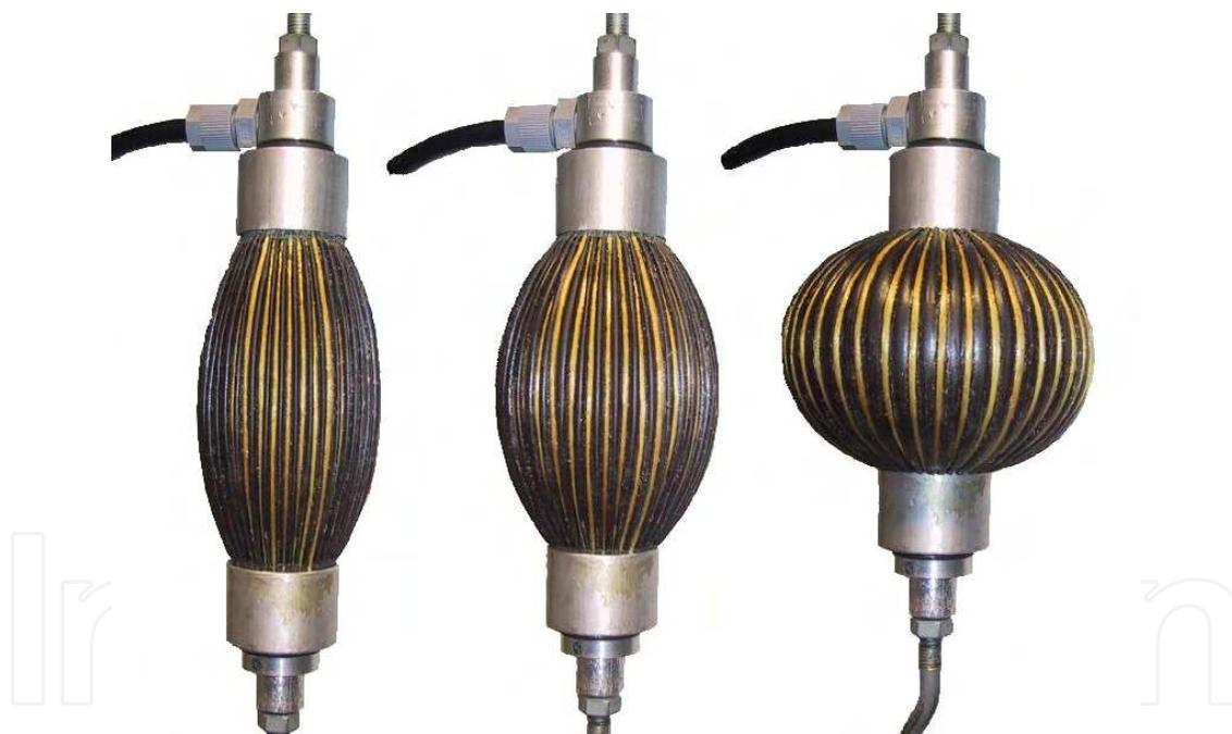
Fig. 1. Pleated Pneumatic Artificial Muscles at 3 different contraction levels.
