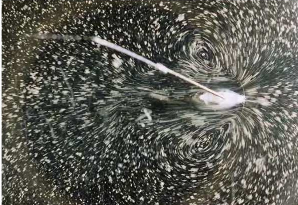
Fig. 20. Flow visualization around a tethered opossum shrimp in dorsal view
