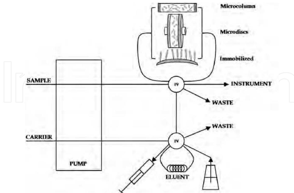
Fig 1. Flow configuration for the use of carbon nanotubes as sorbent in solid phase extraction procedures.
