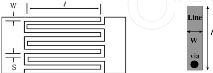
Fig. 2-3. Microstrip interdigital coupled lines and grounded stub
