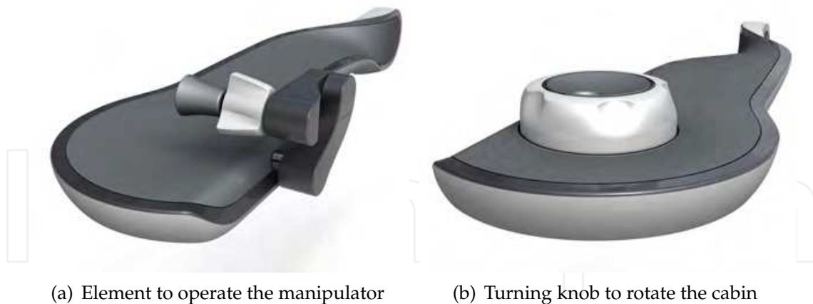
Fig. 4. Enlarged view of the operating elements
