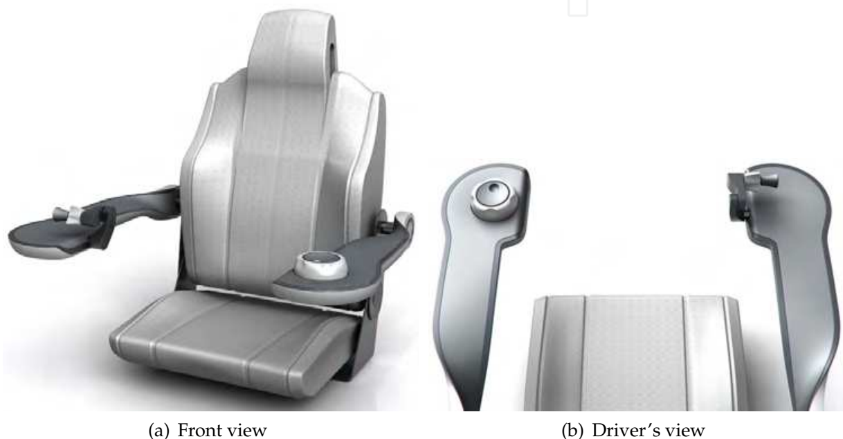
Fig. 3. Intuitive operational concept for hydraulic excavators
