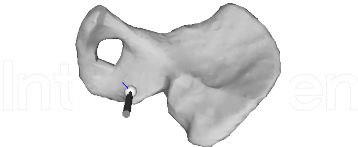
Fig. 12. A burr-tool receiving force-feedback from a polygonized pelvis model where the force (direction and strength) is displayed with a blue line
