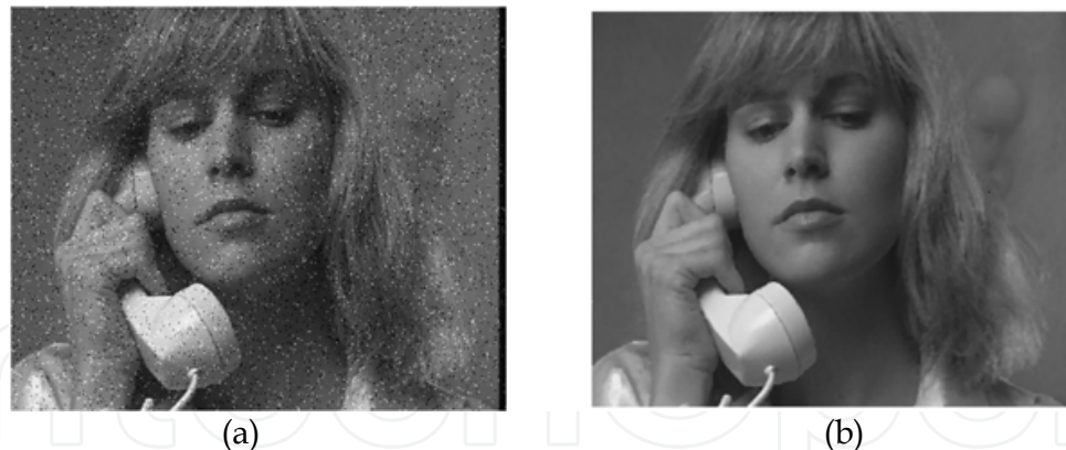
Fig. 3. Two-dimension application of MED filter.
