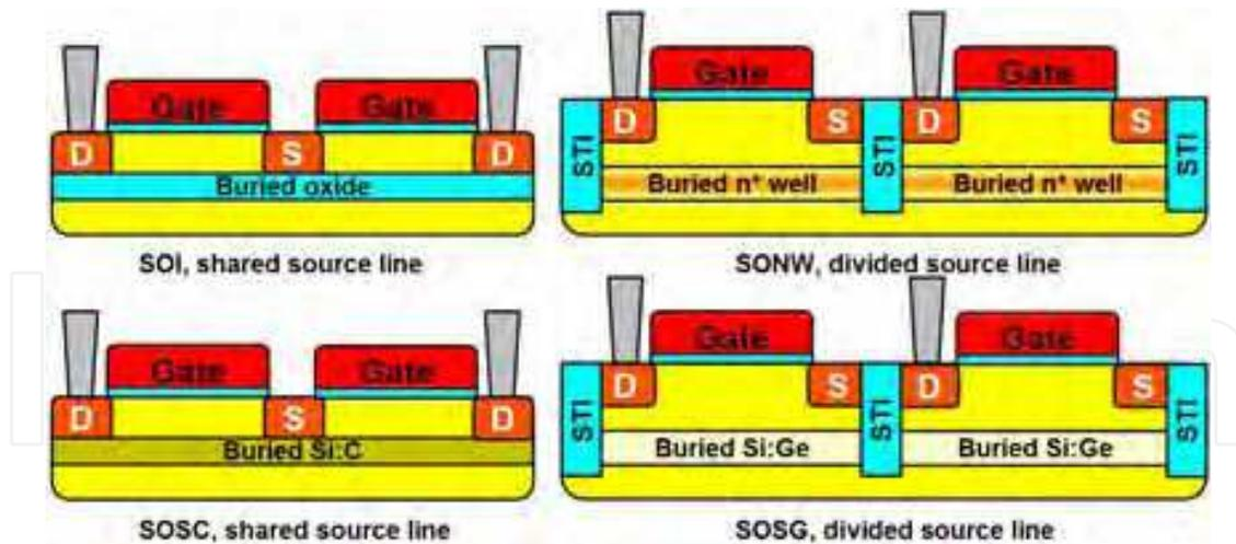
Fig. 3-3. Schematics of the cells along the word line direction. Whereas the SOI and SOSC use the shared bit line, the SONW and SOSG should utilize the divided source line.
