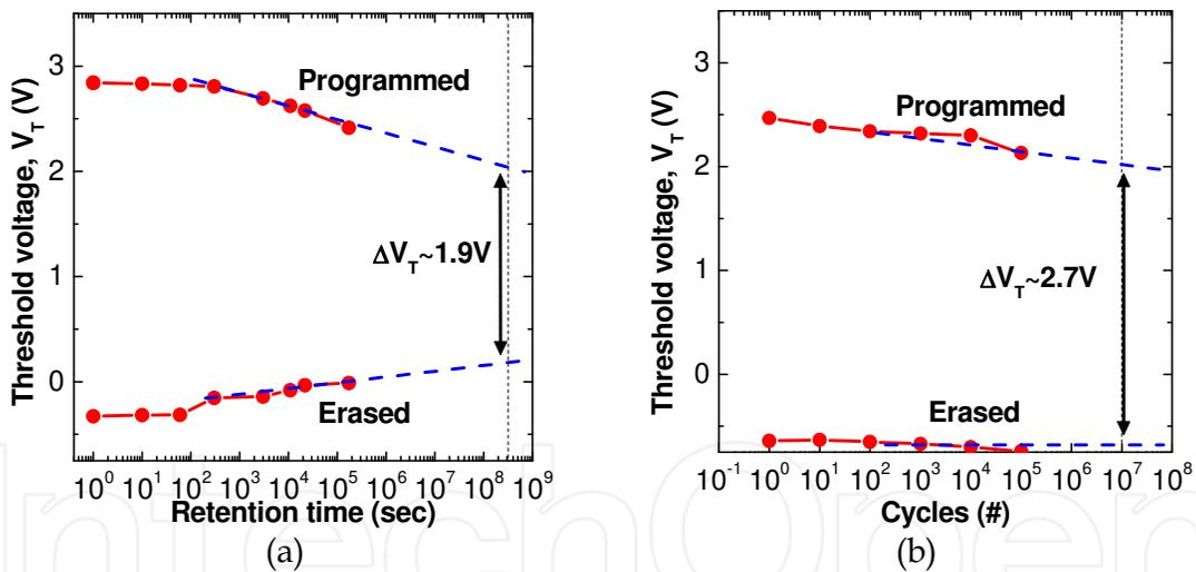
Fig. 4-4. (a) Data retention and (b) endurance characteristics of Flash mode at SOI URAM. (Han et al., 2007)
