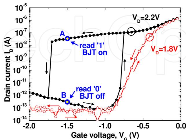
Fig. 5-6. Double sweep drain current versus the gate voltage characteristics at the SOI URAM. At  $V_D=1.8V$ , the device shows normal MOSFET transfer characteristics. At  $V_D=2.2V$ , the parasitic BJT alternatively begins to work, and the hysteresis loop is created.
