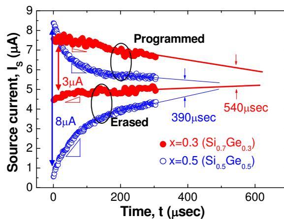
Fig. 4-12. Capacitorless 1T-DRAM characteristics for different germanium content in  $\text{Si}_{1-x}\text{Ge}_x$  of SOSG. The higher  $x$  exhibits a wider sensing window at the beginning of the sensing, but also faster charge loss. (Han et al., 2008b)
