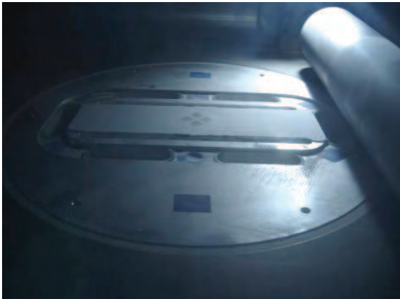
Fig. 1. Selective laser sintering of PLLA/CHAp powder in progress.
