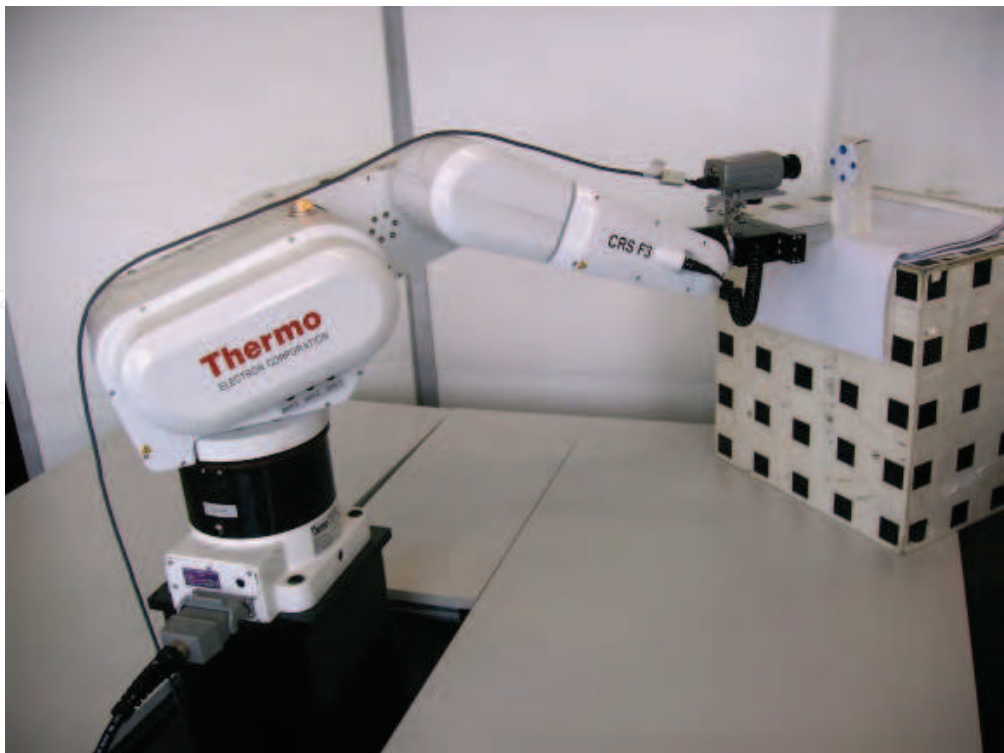
Fig. 11. Experimental setup with Thermo CRS F3 robot, camera and marked object
