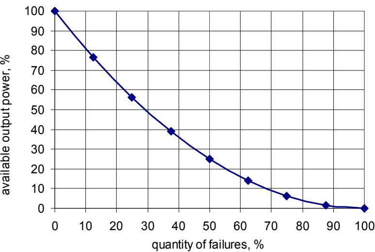
Fig. 3. Combined output power vs number of failed input sources
