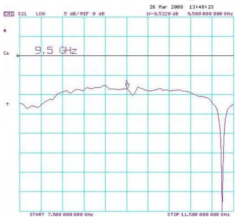
Fig. 15. Example of measurement results – transmission characteristics from centre coax input to one of coax output port
