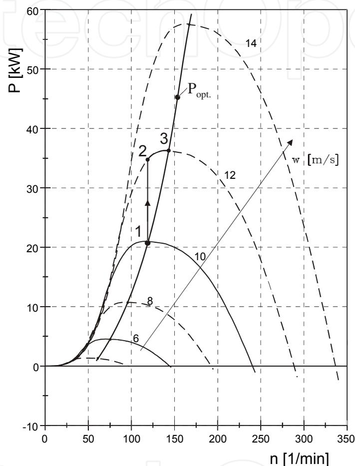
Fig. 2. Power map example of a wind rotor
