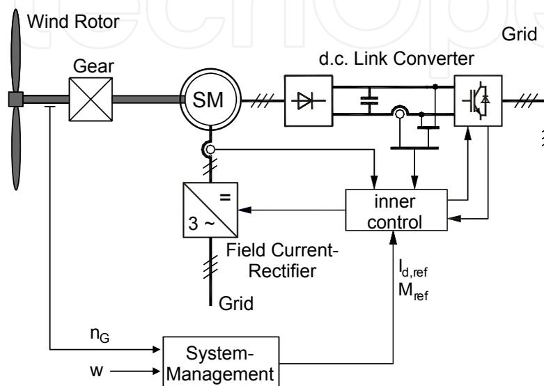
Fig. 9. Operating principle of average value power control
