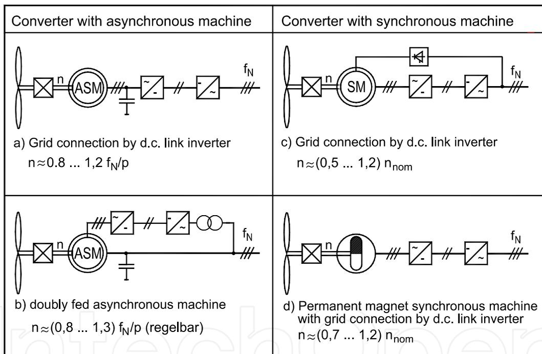
Fig. 1. Applied Generator Systems for variable speed wind energy converters
