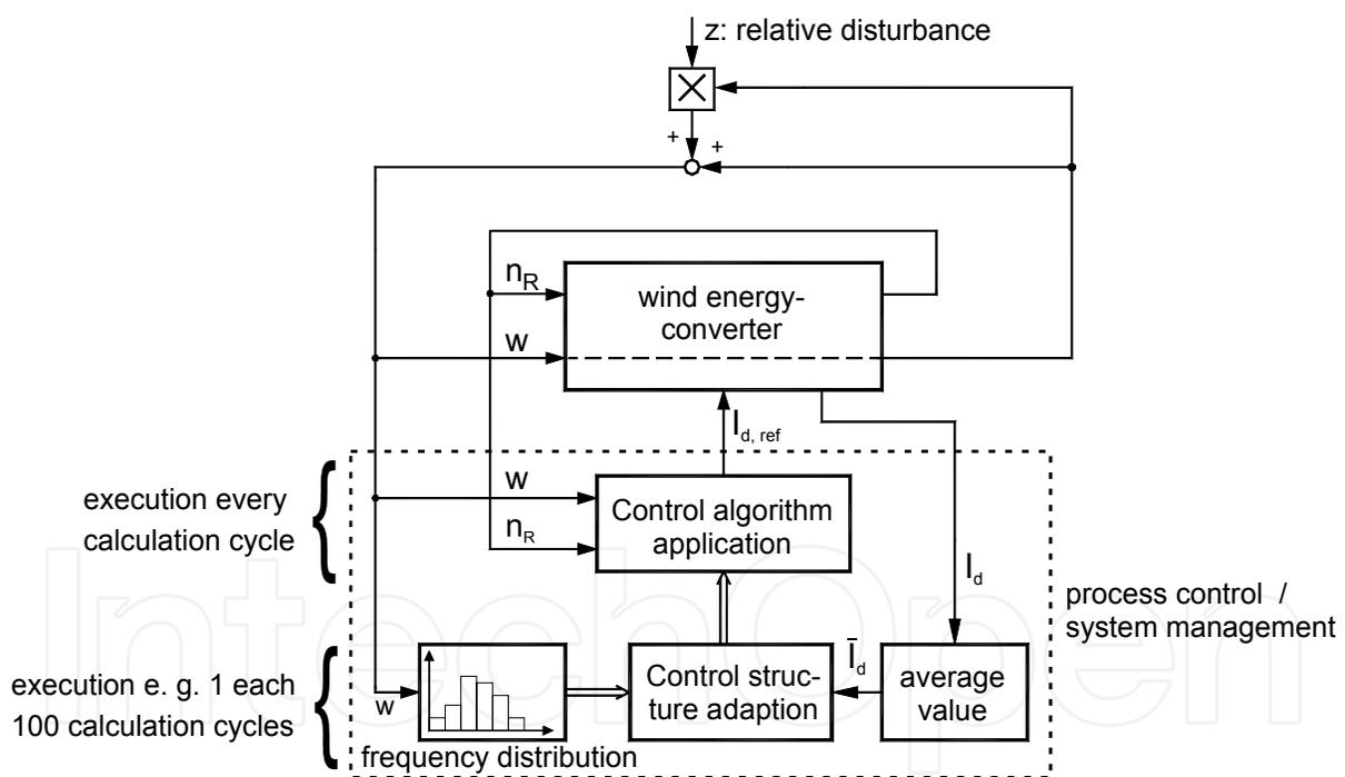
Fig. 11. Block diagram of an iterative self-adapting system management
