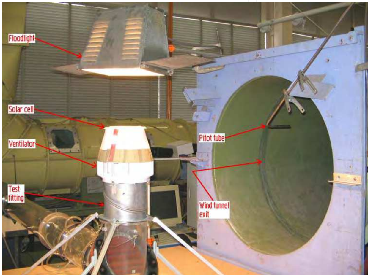
Fig. 12. Test set-up of wind-solar hybrid ventilator
