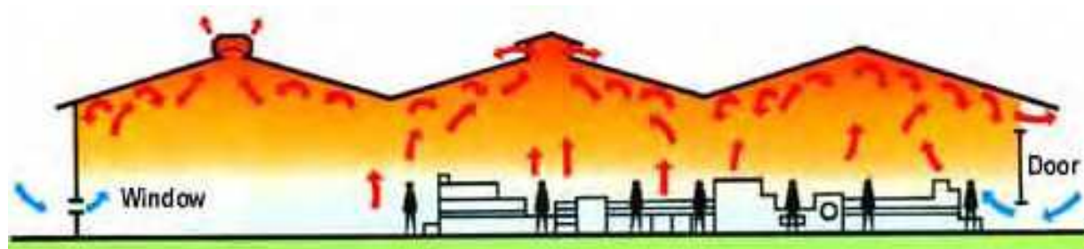
Fig. 1. Ventilation by Natural Convection (Image: www.lomanco.com )
