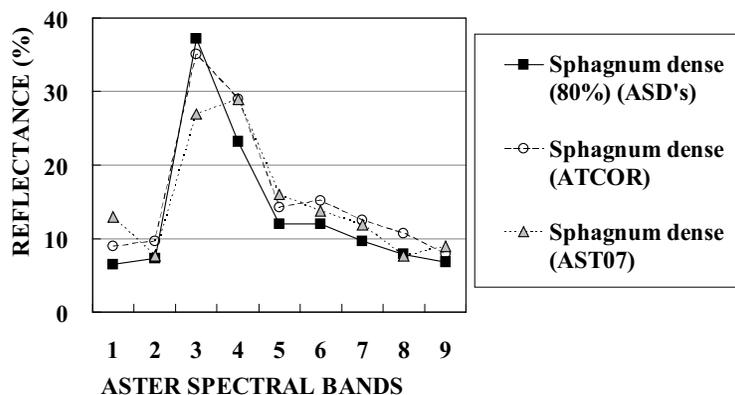
Fig. 3 (2) Comparison of the spectral reflectance of high moor plant *Sphagnum* marsh calculated from ASD's measurement method, ATCOR method and EOSDIS AST07 method.
