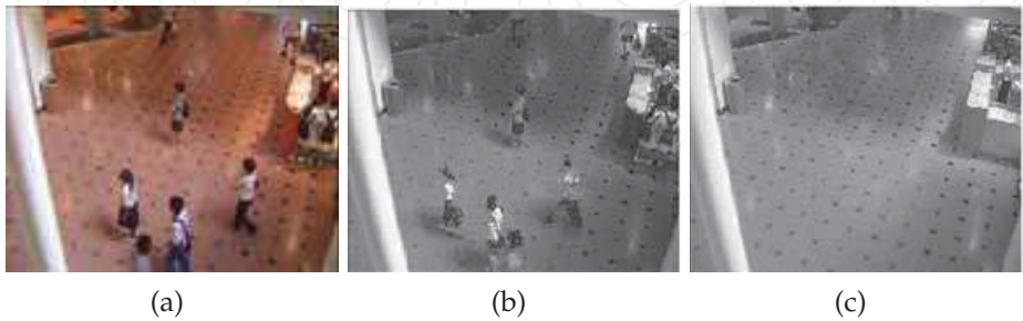
Fig. 11. Non-empty background: (a) Mall video sequence. (b) Background model after 5 frames using the RM method. (c) Background model after 95 frames using the RM method.
