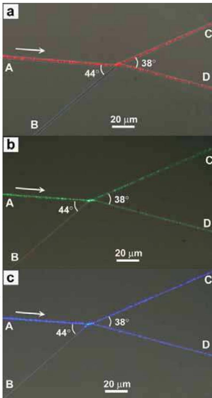
Fig. 22. Optical microscope images of the guided visible lights in the  $2 \times 2$  optical beam splitters with branching angles of  $44^\circ$  and  $38^\circ$ . The diameter of the nanowires is 580 nm. The arrows show the propagation directions of the launched lights with (a) 650 nm red light, (b) 532 nm green light, and (c) 473 nm blue lights.
