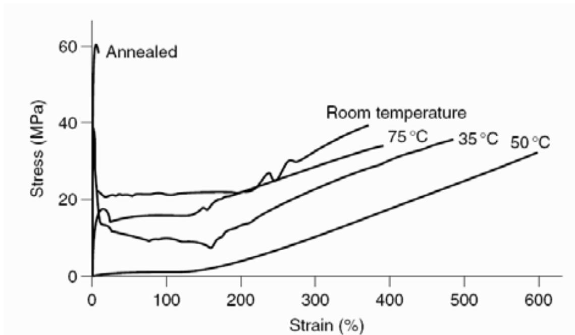
Fig. 5. PTT stress-strain curves at draw temperatures below and above the glass transition temperature [31].
