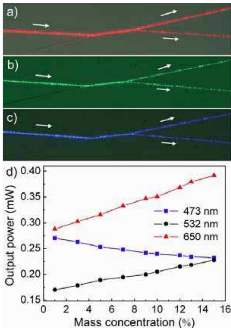
Fig. 36. Optical microscope images of the sensor with (a) red light ( $\lambda = 650 \text{ nm}$ ), (b) green light ( $\lambda = 532 \text{ nm}$ ), and (c) blue light ( $\lambda = 473 \text{ nm}$ ) in it (without sample solution). The white arrows show the propagation directions of the light. (d) Output power in the output branch 1 as a function of mass concentration of solution at branching angles of  $20^\circ$  and light of different wavelengths (473, 532, and 650 nm).
