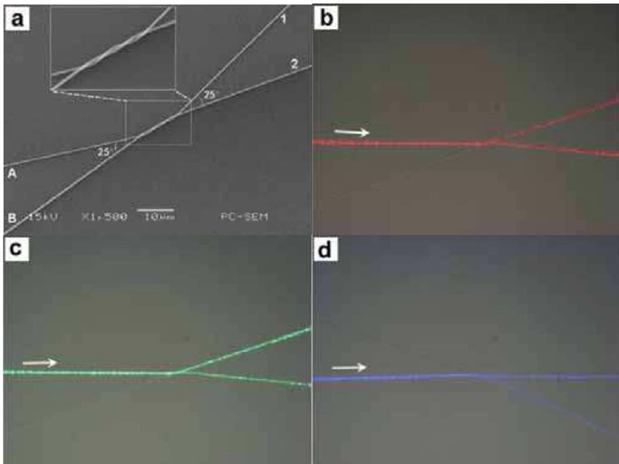
Fig. 20. A  $2 \times 2$  photonic coupling splitter. (a) SEM image of the splitter with diameters of 460 and 548 nm for branches A-1 and B-2, respectively. (b)-(d) Optical microscope images of the guided red (650 nm), green (532 nm) and blue (473 nm) lights, respectively. The arrows show the propagation directions of the launched lights.
