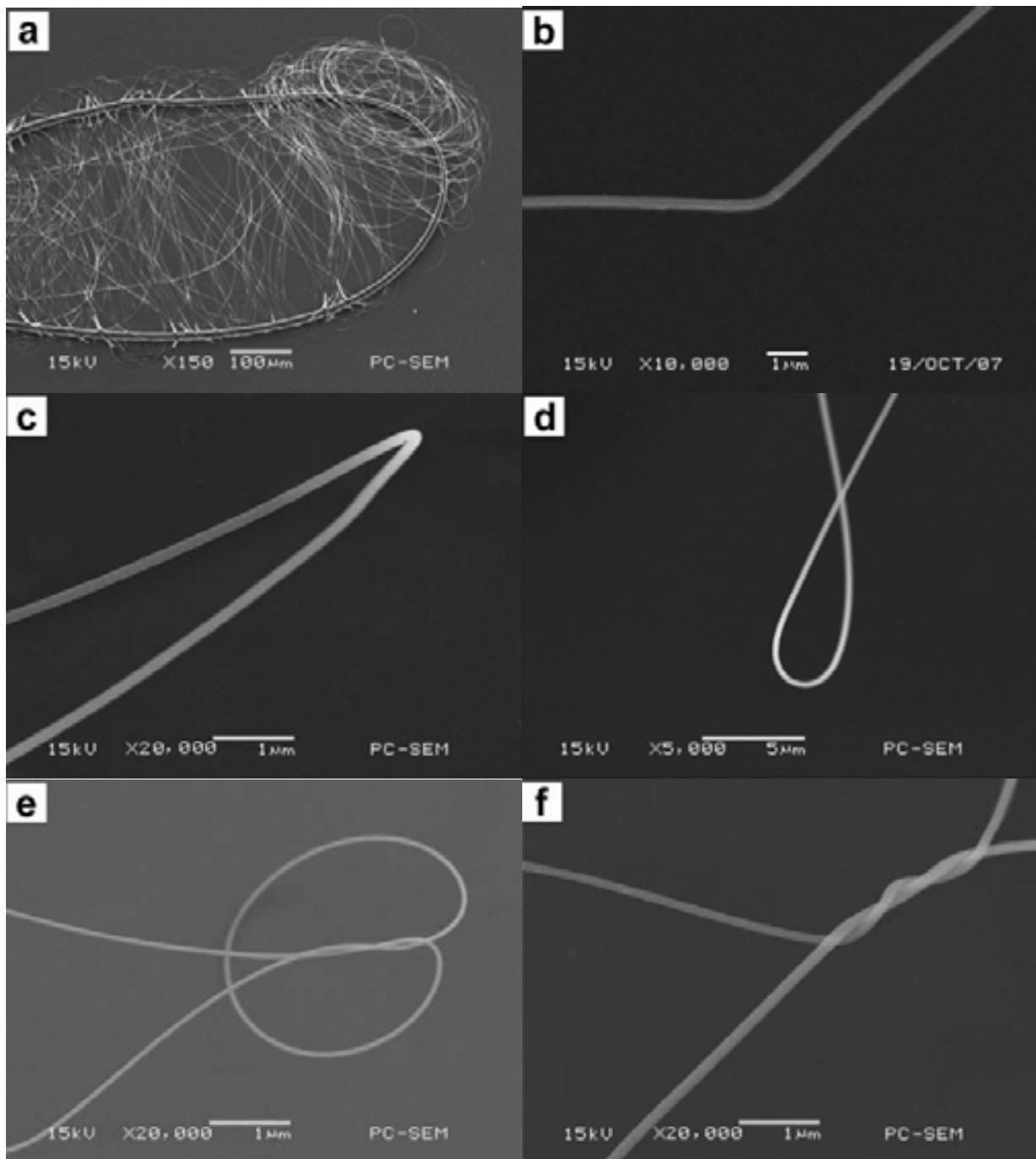
Fig. 17. Scanning electron microscope (SEM) images of nanodevices. (a) A nano bird's nest with average diameter of 280 nm on a 12- $\mu$ m-diameter PTT bending rod (top right). (b) A 45° bend with a diameter of 280 nm. (c) A 155° sharp bend with a diameter of 160 nm. (d) A 340-nm-diameter tweezer-shaped nanowire. (e) A 70-nm-diameter scissor-shaped nanowire. (f) A twisted 2 $\times$ 2 coupler consists of 110-nm- and 150-nm-diameter nanowires.
