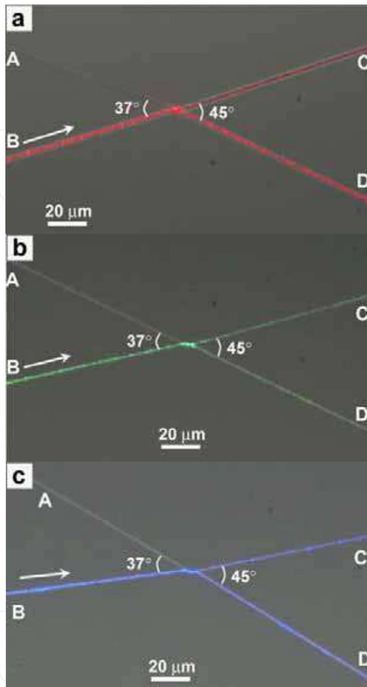
Fig. 21. Optical microscope images of the guided visible lights in the  $2 \times 2$  optical beam splitters with branching angles of  $37^\circ$  and  $45^\circ$ . The diameter of the nanowires is 580 nm. The arrows show the propagation directions of the launched lights with (a) 650 nm red light, (b) 532 nm green light, and (c) 473 nm blue light.
