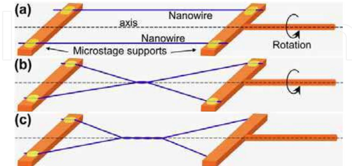
Fig. 16. (a) Two parallel PTT nanowires were fixed by two microstage supports. The left support is fixed and the right support can be rotated around the axis. (b) A twisted  $2 \times 2$  structure with one twisted turn was formed by rotating the right support. (c) A twisted  $2 \times 2$  structure with four twisted turns was formed by further rotating the right support.
