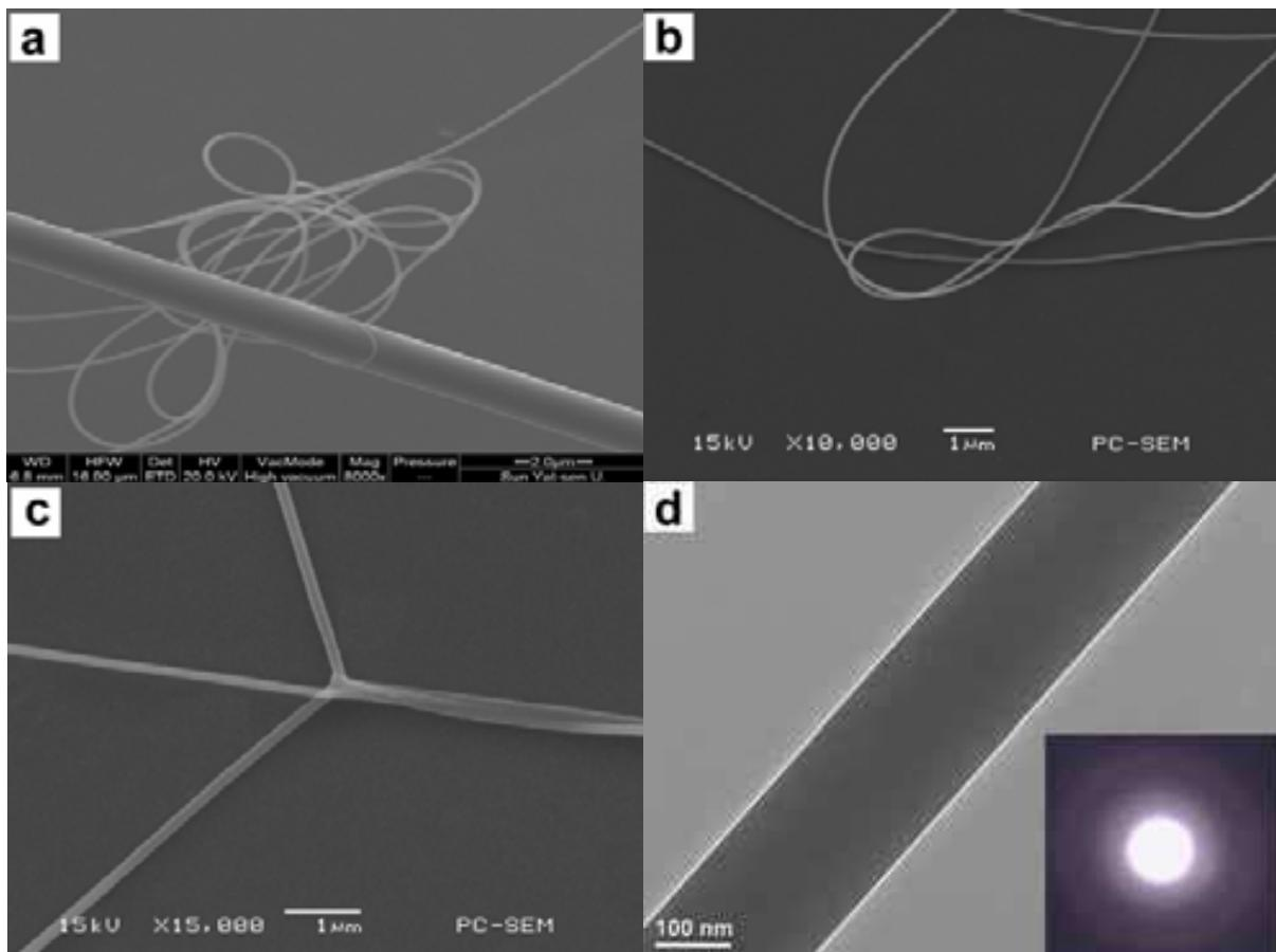
Fig. 9. Electron micrographs of PTT nanowires and nanowire structures. a–c, SEM images: (a) Comparison of a 167-nm-diameter PNW (about 155  $\mu\text{m}$  long) with a 1.26- $\mu\text{m}$ -diameter straight PTT rod. (b) Four 110-nm-diameter PNWs are positioned together. (c) Flexible and elastic enough PNWs connection with diameters of 140 and 170 nm. (d) TEM image of a 190-nm-diameter PNW. The inset shows its electron diffraction pattern.
