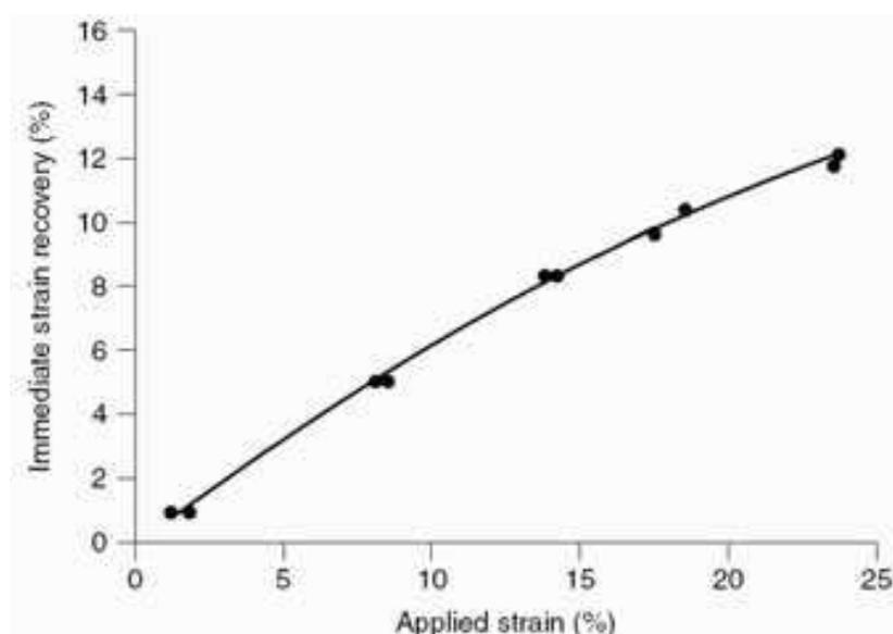
Fig. 3. PTT elastic recovery at various strains [26]
