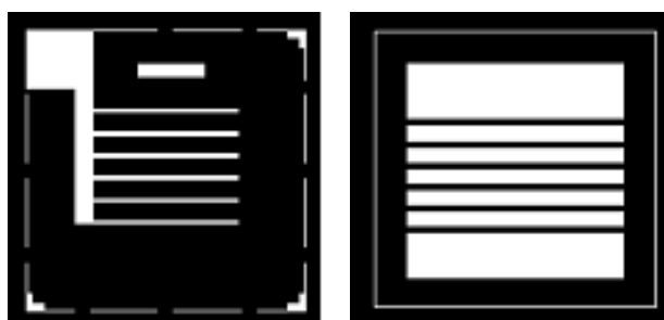
Fig. 10. Masks of device fabrication by MIMIC process.
