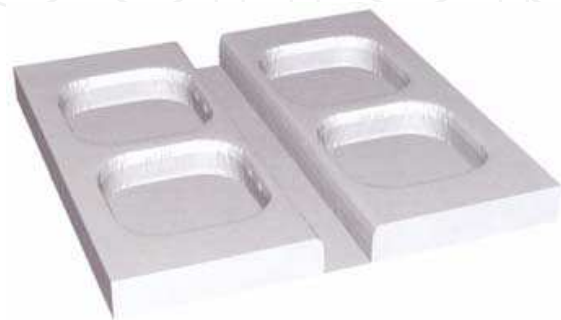
Fig. 20. Simulated 3D resist profiles for a layout consisting one 30 nm wide line and four 800 \times 800 \text{ nm}^2 squares at 50 keV e-beam
