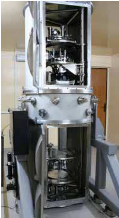
Fig. 16. Photograph of the vertical vacuum interferometer.
