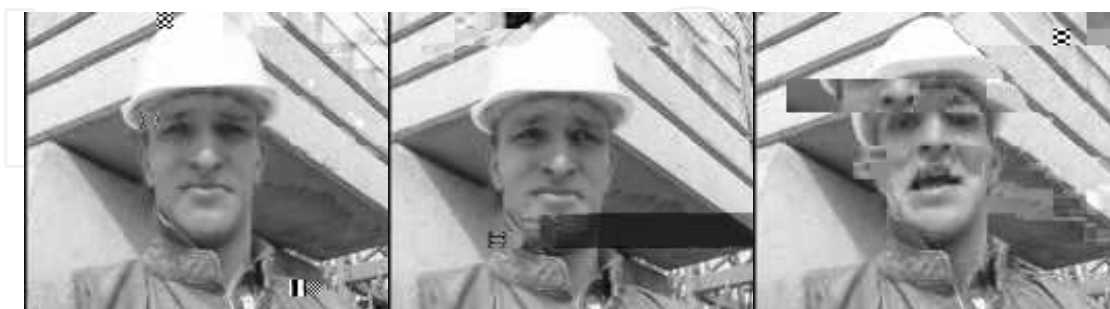
Fig. 4. Examples of visual impairments due to transmission errors ( Foreman sequence, MPEG-2, QCIF@128Kbps, BER = 10^{-4} )
