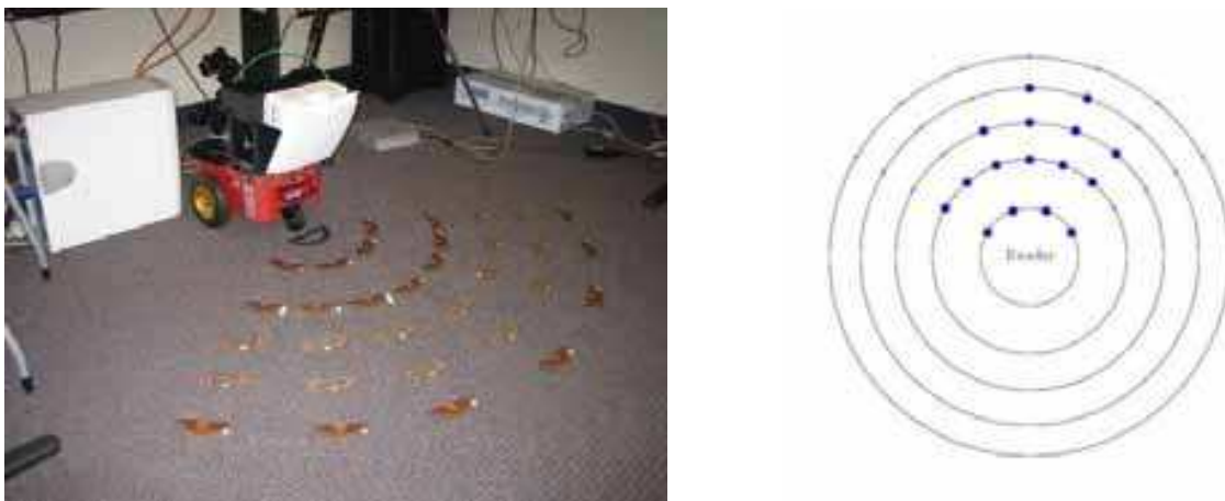
Fig. 10. Left: documentation of setup used to build the sensor model. Right: Image showing nominal detection range when Tags are distributed on the floor and the Reader is mounted on the robot and tilted forward 30 degrees. The 4th "row" has a radius of rough
