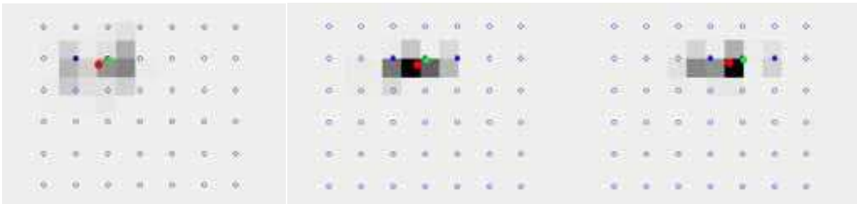
Fig. 12. These images show three time steps in the middle of an experimental run. Open circles represent undetected tags. Filled blue circles represent detected tags. The red circle represents the average robot location, and a green circle represents a ground
