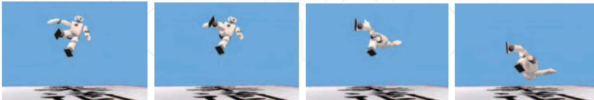
Figure 2. An example of an evolved jump from a reduced gravity run
