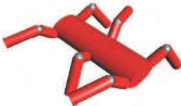
Figure 8. A six-legged body composed of a central body and 12 spherical joints
