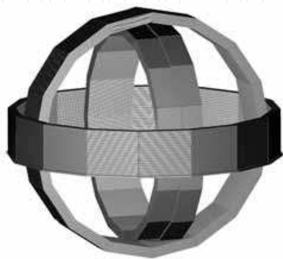
Fig. 14. 3D antenna model for FastHenry simulator
