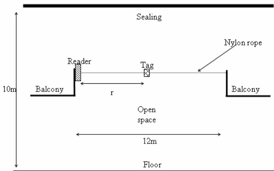
Fig. 5. Setup for determining maximum RFID read distance.
