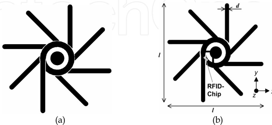
Fig. 13. (a) The Precisia LLC company logo and (b) the same logo changed into an RFID tag antenna.
