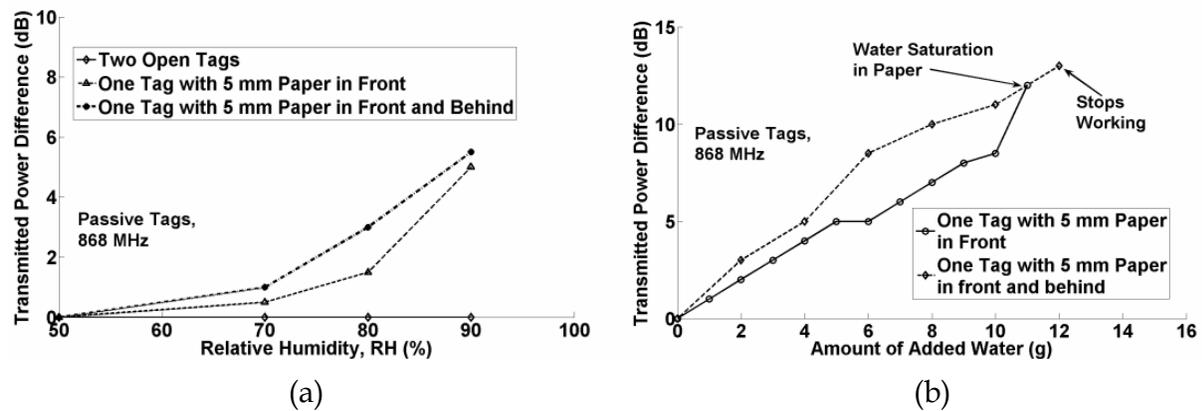
Fig. 17. Difference in minimum output power required from the RFID reader in order to read two passive tags in a label where one is covered or embedded in a moisture absorbing material.
