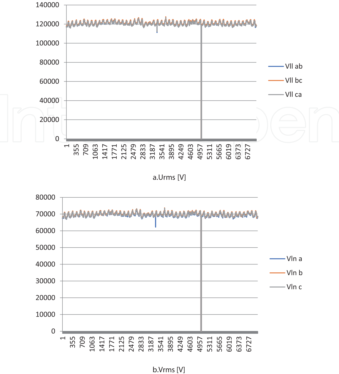
Figure 4. Voltage curve at the supply bar for TGD: a - voltages between phases, b - voltages per phase.
