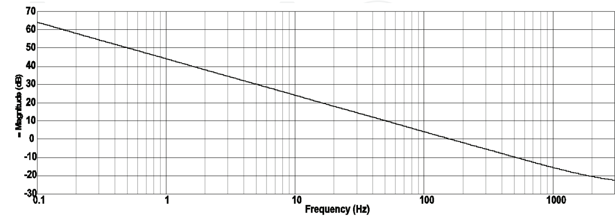
Fig. 19. Frequency response of the integrator circuit. Next section an important application of the op-amp that is an active filter in the physical domain is proposed.
