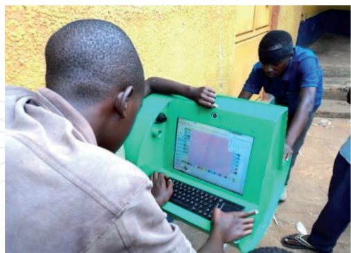
Figure 5. The “Digital Drum” solar-power computer kiosk in Uganda [14].
