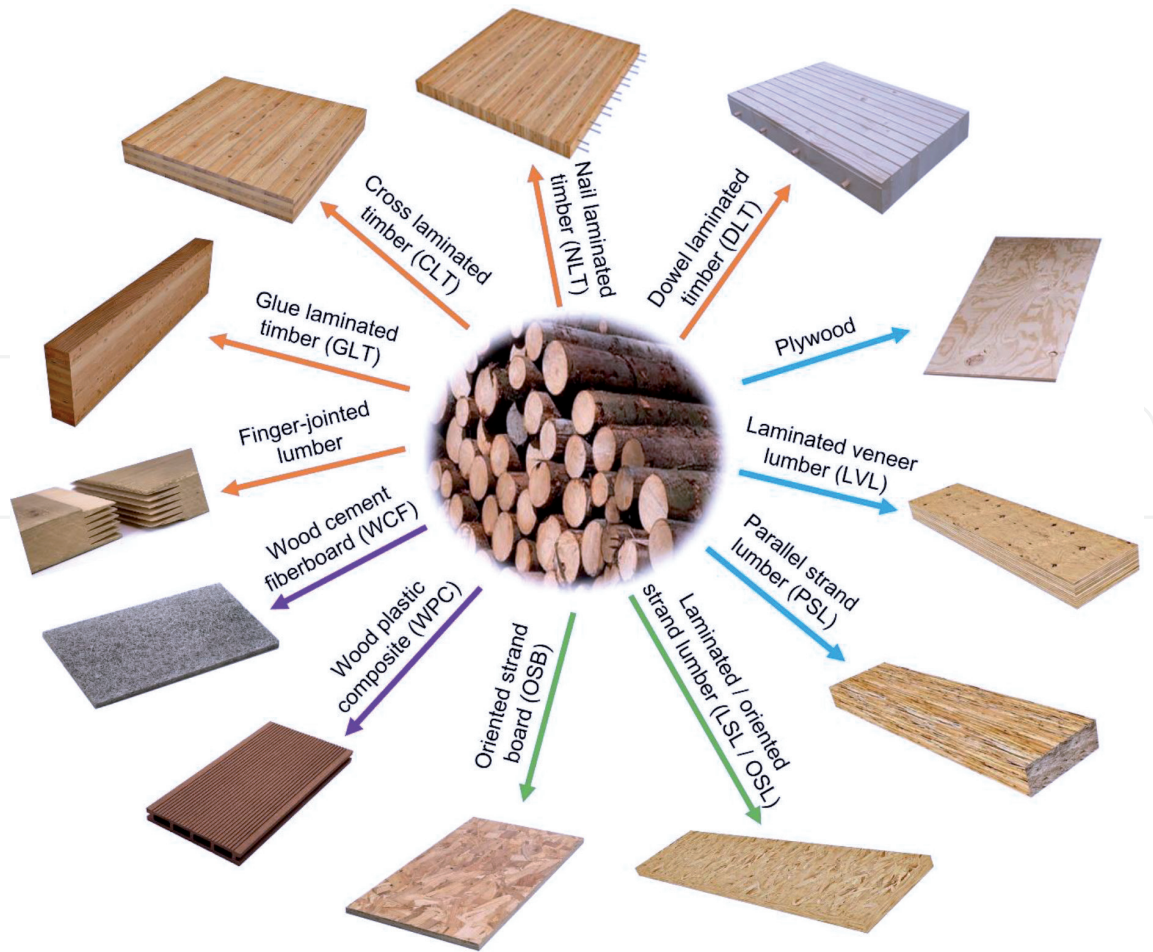
Figure 1. Major types of engineered wood products and their abbreviations (source: images obtained from archiproductions.com, canac.ca, diy.com, globalsources.com, leben.co.in, nrcan.gc.ca, and structurecraft.com).
