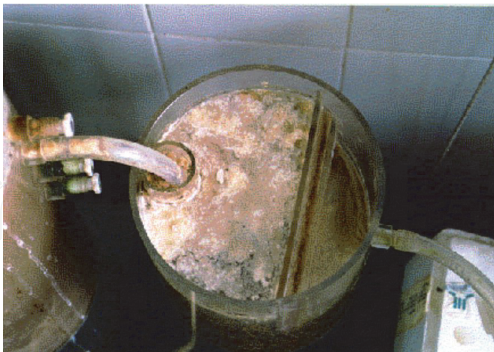
Figure 3. Oil and grease accumulated in settling tank.
