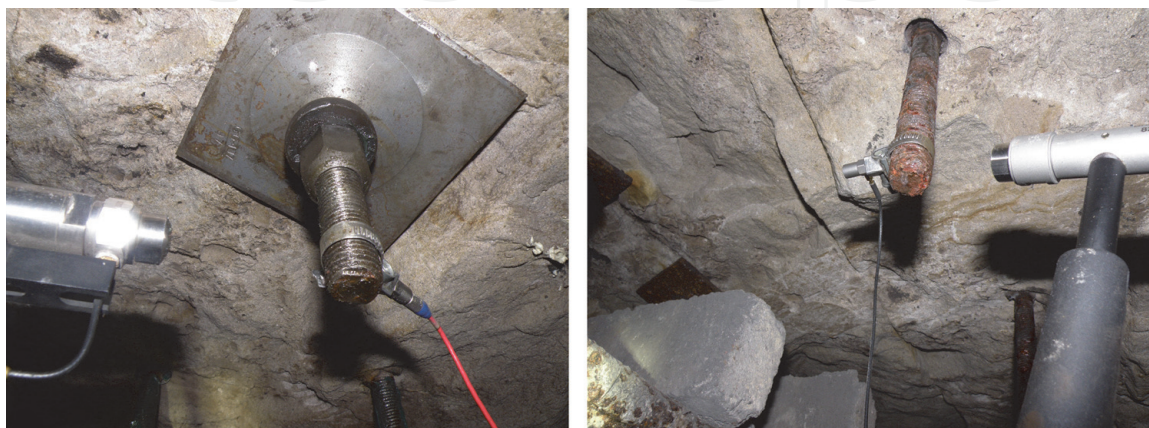
Figure 9. Impact excitation of installed rock bolts, with the working prototype (left) and the unit fulfilling ATEX requirements (right).
