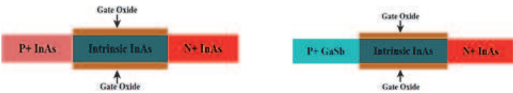
Figure 9. Homojunction and heterojunction TFET using III-V materials.
