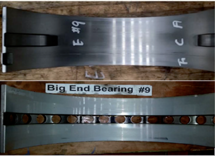
Figure 19. Big end bearing of medium-speed diesel engine.
