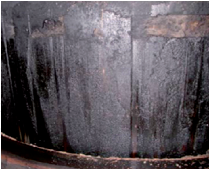
Figure 25. CaCO 3 deposits on the piston top.
