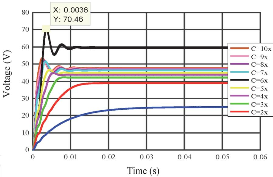
**Figure 16.** CPV system output voltage under the concentration conditions at a constant temperature (35°C) and with FL control.
