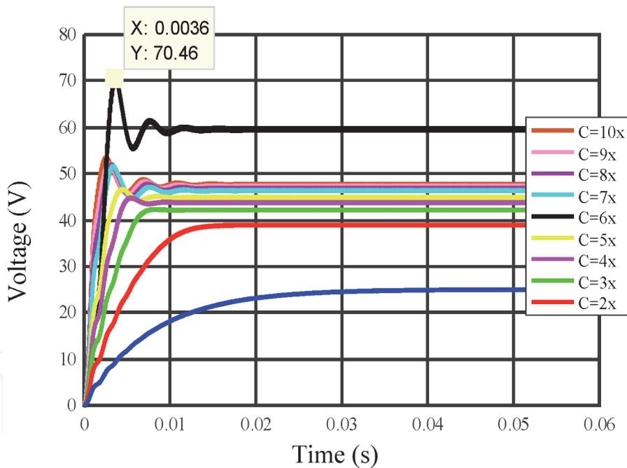
**Figure 13.** CPV system output voltage under the concentration conditions at a constant temperature ( $35^{\circ}\text{C}$ ) and with  $P\&O$  control.
