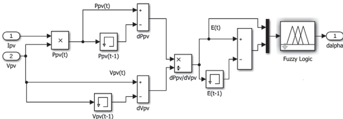
Figure 5. Fuzzy logic algorithm in MATLAB/Simulink®.
