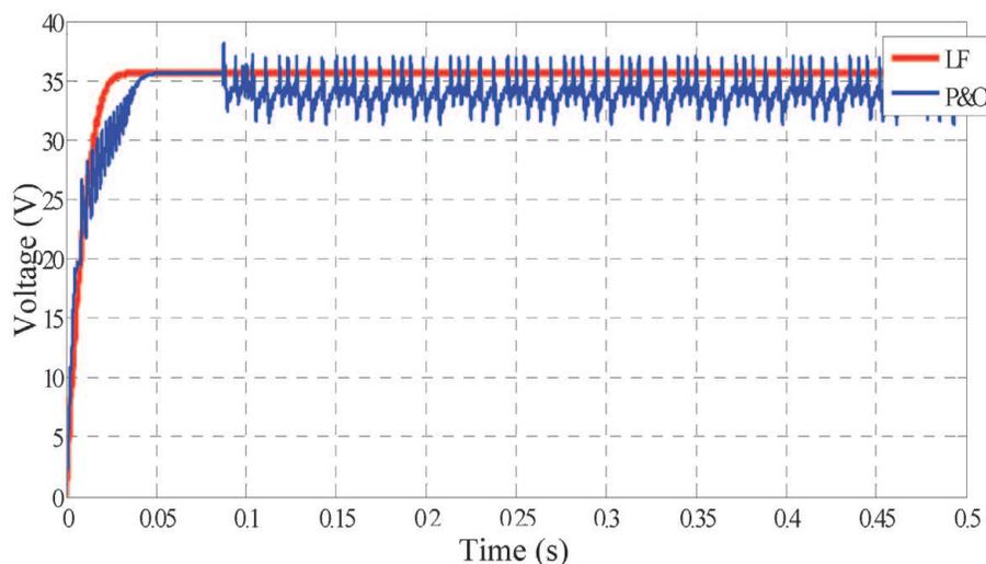
**Figure 6.** Output voltage using the MPPT control (P&O and FL) for  $C = 1x$  and  $T = 53.75^\circ\text{C}$ .
