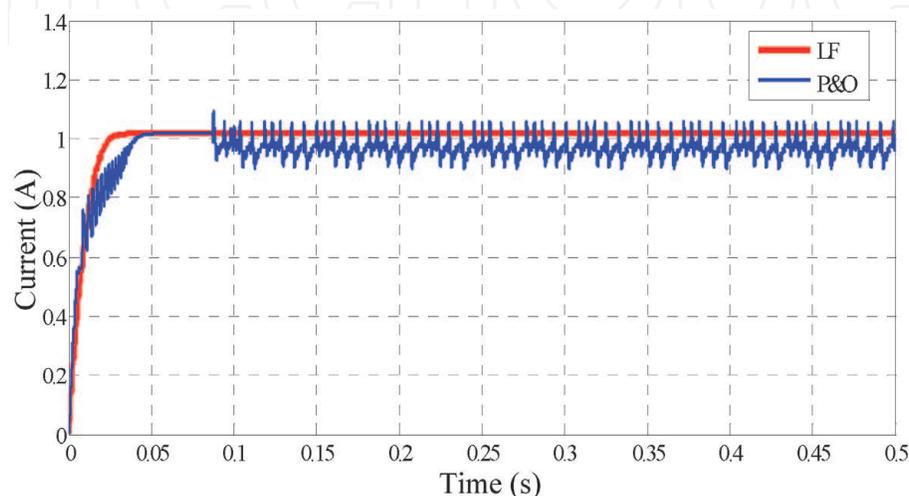
**Figure 7.** Output current using the MPPT control (P&O and FL) for  $C = 1x$  and  $T = 53.75^\circ\text{C}$ .
