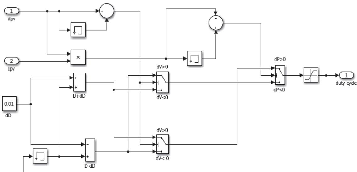
Figure 4. P&O algorithm in MATLAB/Simulink®.
