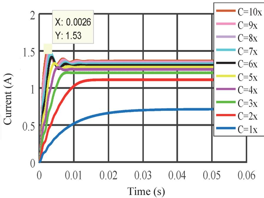
**Figure 12.** CPV system output current under the concentration conditions at a constant temperature ( $35^{\circ}\text{C}$ ) and with  $P\&O$  control.
