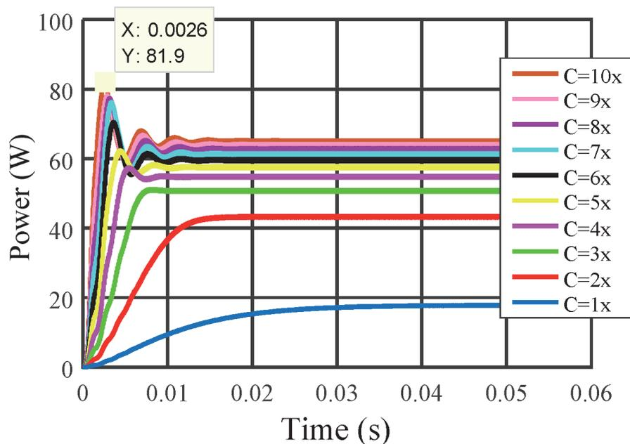
**Figure 14.** CPV system output power under the concentration conditions at a constant temperature (35°C) and with FL control.
