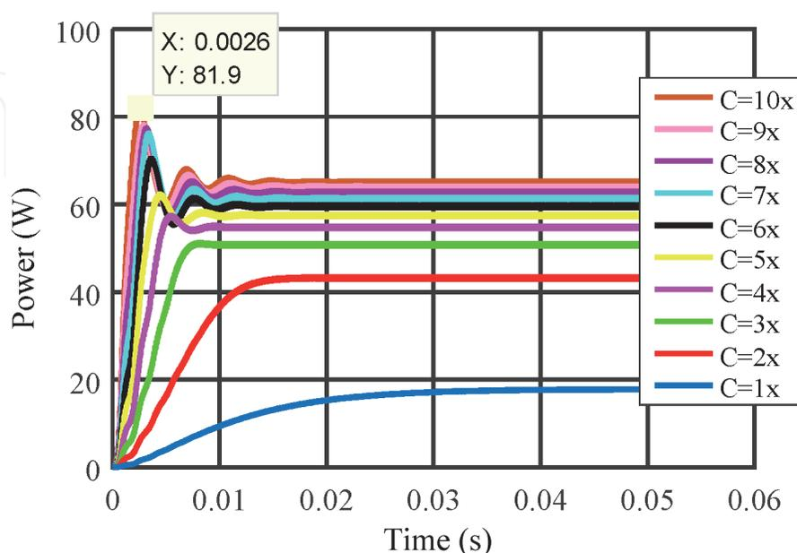
**Figure 11.** CPV system output power under the concentration conditions at a constant temperature (35°C) and with P&O control.
