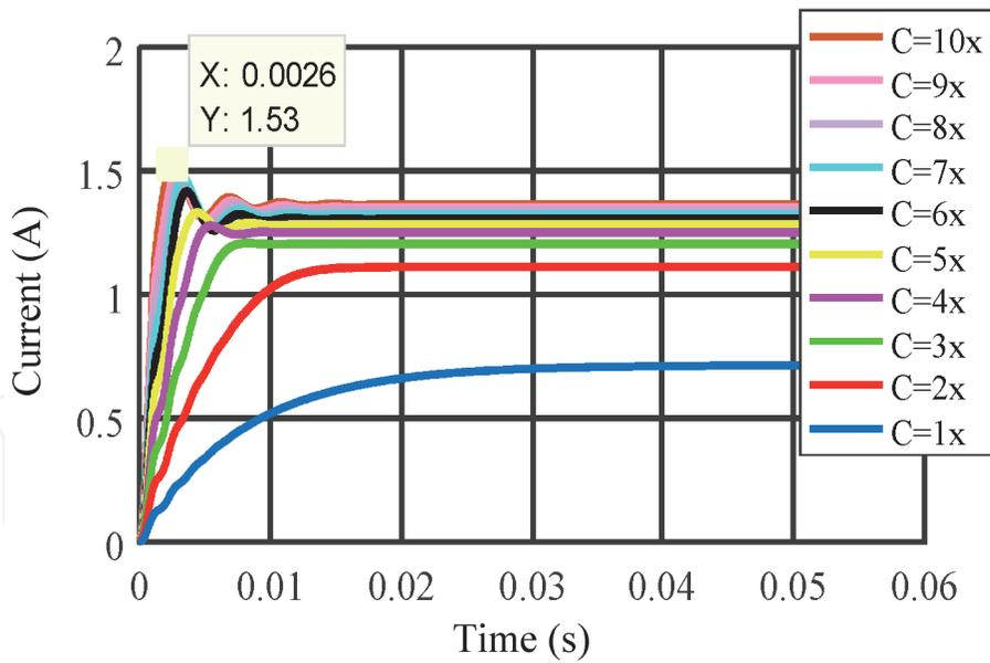
**Figure 15.** CPV system output current under the concentration conditions at a constant temperature (35°C) and with FL control.
