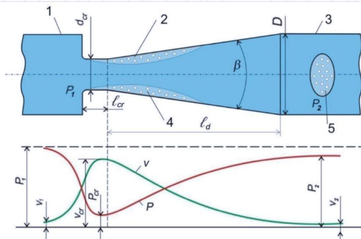
**Figure 2.** Scheme of the cavitation flow in the generator with pressure and flow velocity distribution along the generator length. 1 is inlet pipeline; 2 is generator; 3 is outlet pipeline; 4 is cavitation zone with cavity volume  $V$ ; 5 is detached part of the cavity  $V_2$ ;  $P_1$  is total pressure at the cavitation generator inlet;  $P_2$  is full back pressure.
