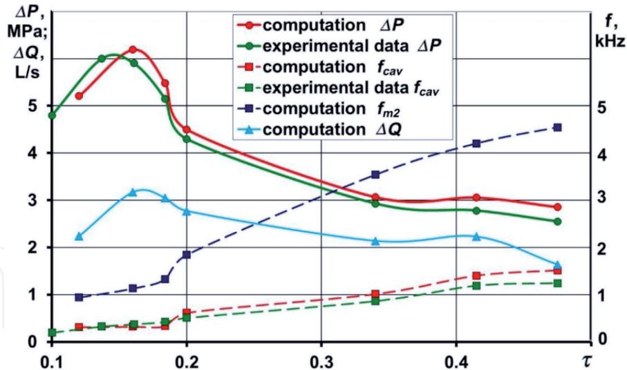
**Figure 9.** Calculated and experimental pressure oscillations range  $\Delta P$ , volumetric flow rate  $\Delta Q$  and hydraulic oscillations frequency  $f$  in the drill bit section vs. the cavitation parameter  $\tau$ .
