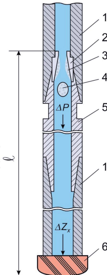
**Figure 1.** Layout of a drill string with a cavitation hydraulic vibrator. 1 is drill pipe; 2 is cavitation generator; 3, 4 are the cavity is sedentary and its cavity part that has come off; 5 is hydraulic vibrator; 6 is drill bit.
