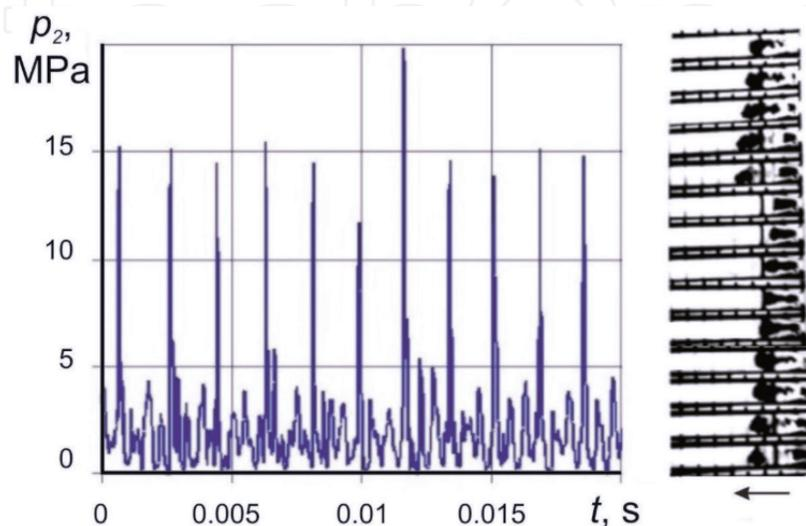
**Figure 3.** Fragment of the oscillogram recording the pressure  $p_2$  in time at the cavitation generator output with the critical section diameter  $d_{cr} = 6$  mm at  $\tau \approx 0.1$  and a filmogram of the growth and separation of the cavitation cavity in the generator tube (the direction of fluid flow is indicated by an arrow).
