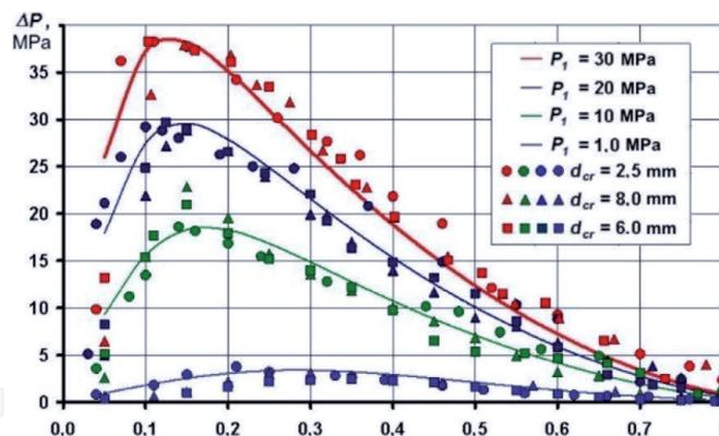
**Figure 4.** Theoretical and experimental dependences of the amplitude  $\Delta P$  of pressure oscillations on the cavitation parameter  $\tau$  realized by the cavitation generator for case of the inlet pressure  $P_1$  changes from 1 MPa to 30 MPa.
