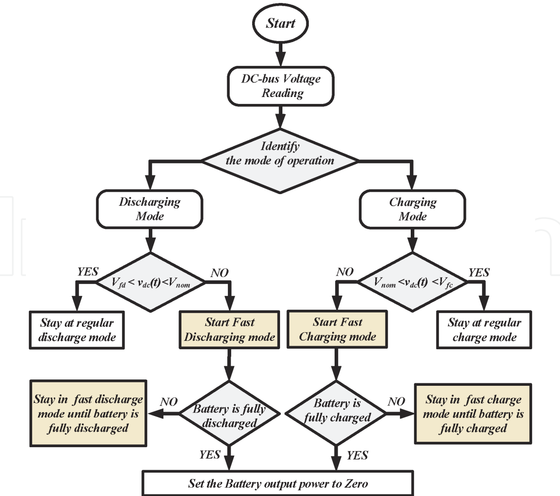
Figure 8. The flowchart of the proposed control scheme for the ESS.
