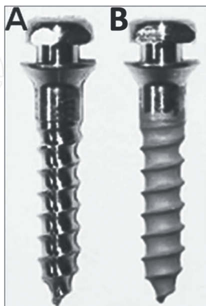
Figure 5. Surface modification by anodic oxidization. (A) Machined surface miniscrew; (B) Anodic oxidized miniscrew. (Taken from: Choi et al. [44].)
