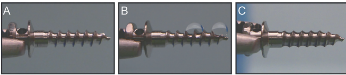
Figure 9. Hydrophilic conversion by photofunctionalization: (A) miniscrew; (B) untreated miniscrew with 2 drops ( 1 \mu\text{L} each); (C) photofunctionalized miniscrew with 2 drops (Taken from: Tabuchi et al. [103].)
