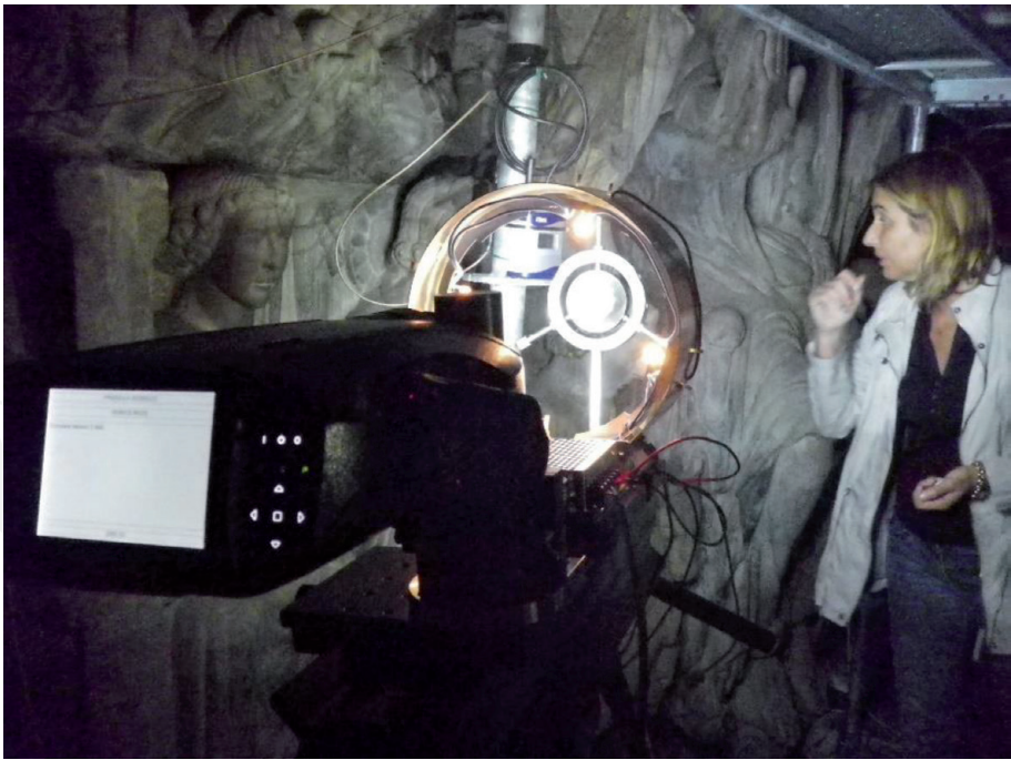
Figure 2. Spectroradiometer with standard white at Pórtico de la Gloria.
