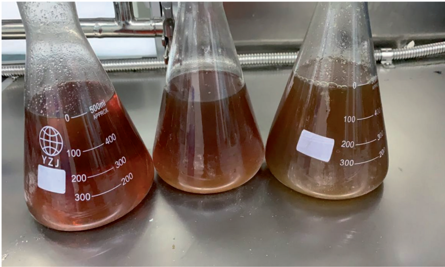
Figure 5. The pyrolysis oil of PP plastic granules.
