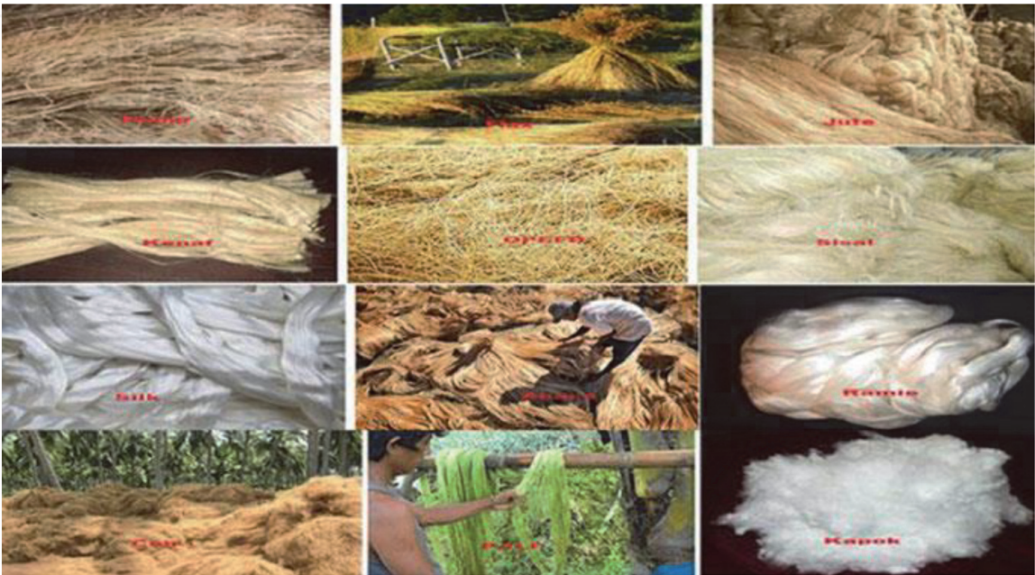
Figure 3. Different types of natural fibers used as reinforcement in polymer composites.
