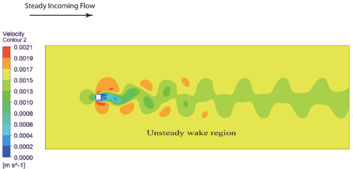
Figure 1. Unsteady wake region, even though oncoming flow is steady state.
