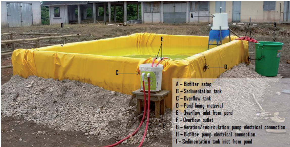
Figure 4. Parts of a typical recirculating aquaculture setup.
