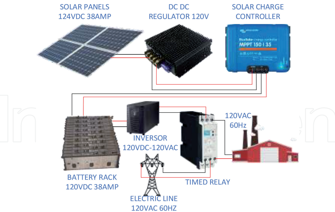
Figure 8. Laboratory power configuration with battery packs.
