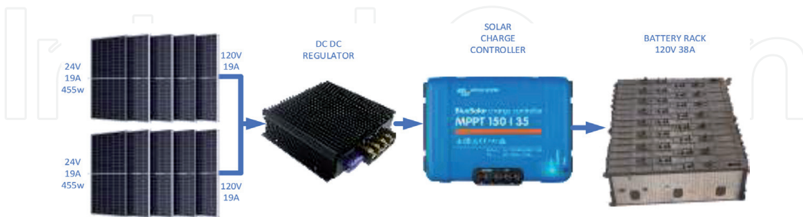
Figure 15. Components of the solar powered charging unit.
