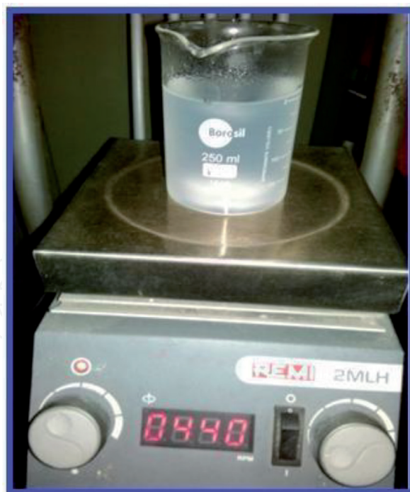
Figure 2. Zinc chloride solution is heated on a magnetic stirrer at speed 450 rpm upto 70°C.
