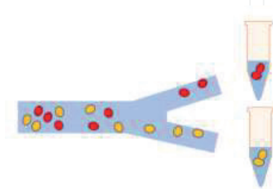
Figure 5. A generic microfluidic channel with 2 outputs. The process for selecting one or another population depends on the nature of the chip. Several different techniques have been demonstrated.
