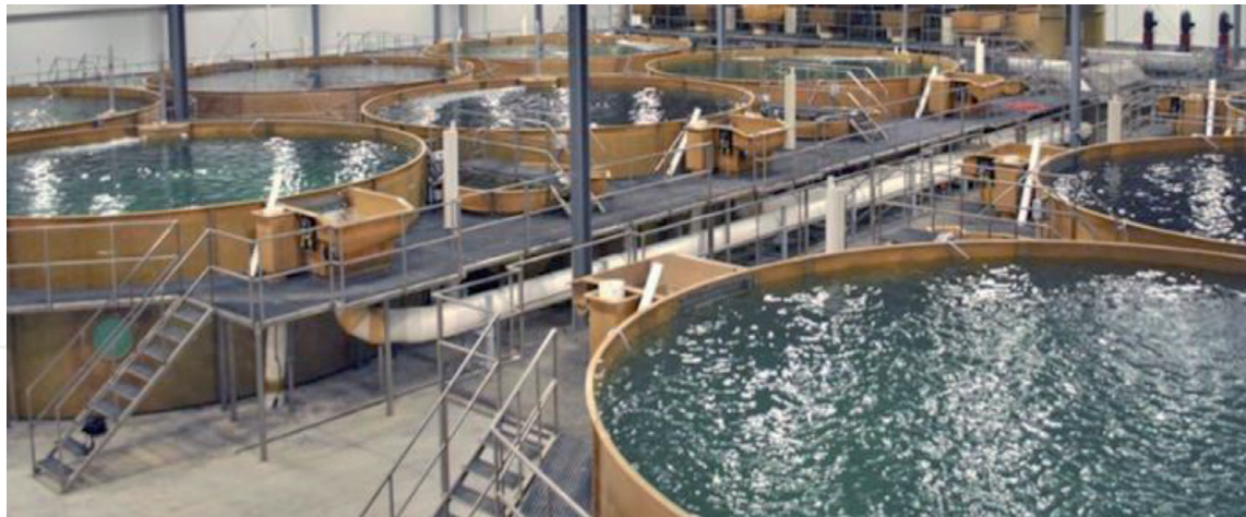
Figure 11. A recirculating aquaculture system.
