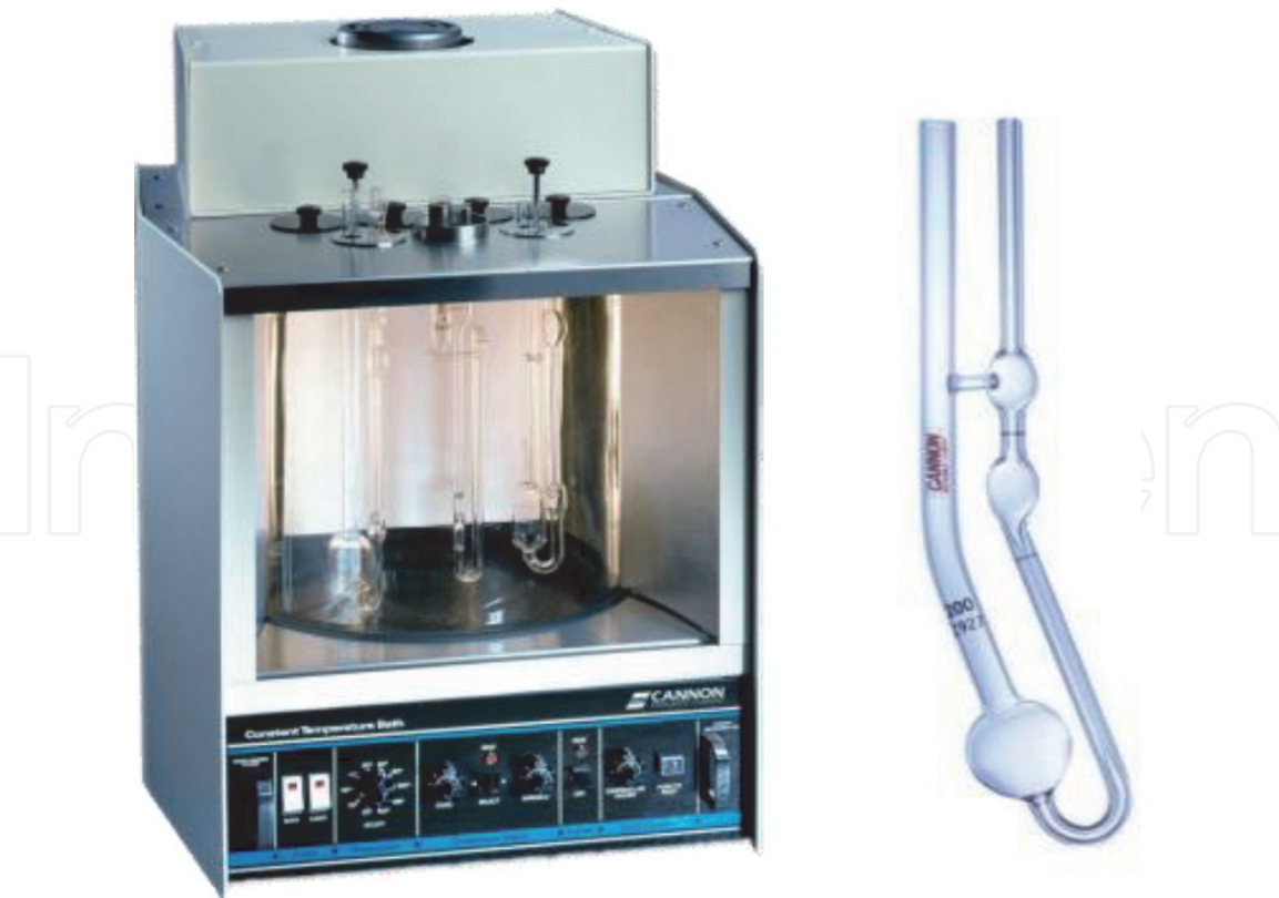
Figure 6. Cannon-Fenske apparatus used for viscosity measurement.
