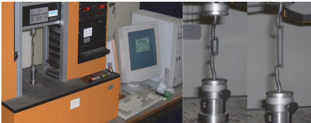
Figure 3. Tensile test setup using elastomer ring samples; different stages of testing.
