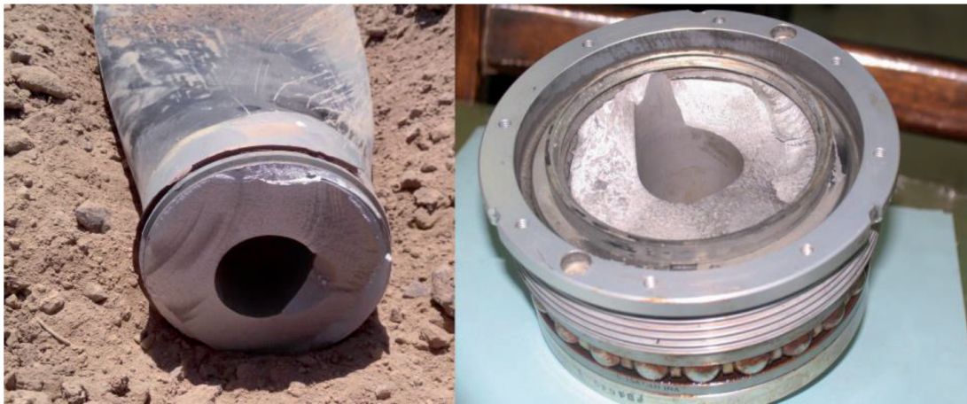
Figure 1. Fatigue failure of bonanza F33 propeller.
